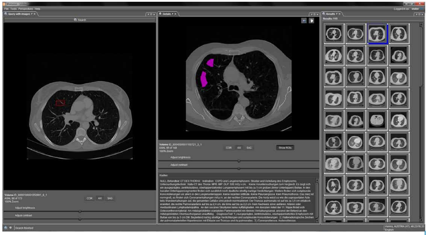
The Khresmoi Radiology Prototype, showing the query case (left) and search results (right) together with the selected search result image (centre) and corresponding radiology report data.
